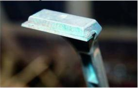
This type of scraper uses a reversible tungsten-carbide blade. It was so sharp it shaved the paint off unless you got the blade right underneath the paint layer, and its uber-sharp edges had a tendency to bite into the paint.
