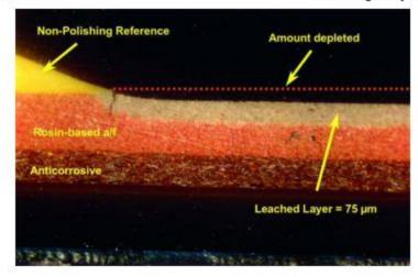
This magnified image is a cross-section of a self-eroding antifouling paint.
