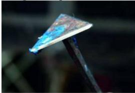
Sharpened on a grinding wheel and with its pointed corners ground off, it made light work of 21 years' worth of paint. An advantage is that you have three scraping surfaces to work with, which gives you extra time before it needs sharpening with a file - which needed doing frequently.
