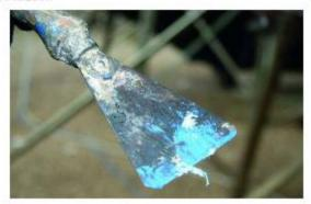
This, sharpened on a grinding wheel and with the corners ground off, was good for lifting flakes of paint off. But for heavy-duty scraping it had a tendency to dig in and try to gouge the gel coat.
