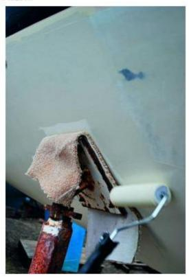
I keep my boat on a trailer over the winter and, impatient to get the job done, I chocked the boat up with a hefty fence post, plywood squares and wedges, before gingerly lowering and removing the pad. I painted underneath the pad, ran out of time and wound it back up too soon.
