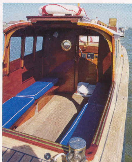
The boat's teak deck was completely relaid and the hardware revitalised; the guest cockpit area (above) with its distinctive trio of windows
