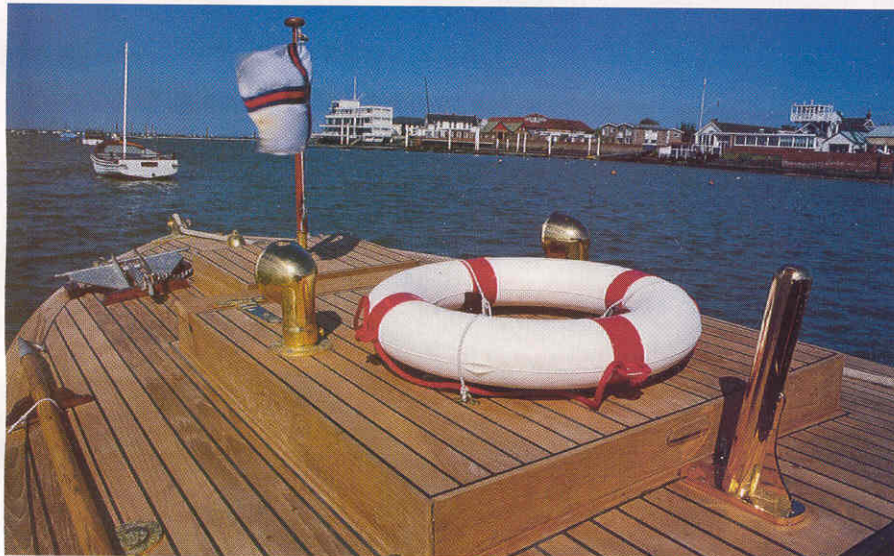
The boat's teak deck was completely relaid and the hardware revitalised; the guest cockpit area (above) with its distinctive trio of windows
