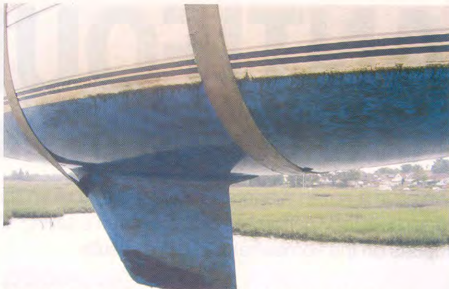
Meltemi III at season's end. The hull looks fouled but the slime came off with ease
