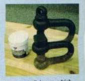
friendly. The molecules of the paint incorporate linkages, which lock them onto rust and combine them with the coating, preventing further degradation.
