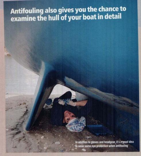
boats in mud berths. The toxic properties of the paint are tightly packed into a hard layer, which remains once the toxins have been exhausted. After several years of recoating, the build-up needs to come off – which can be messy and time consuming.
