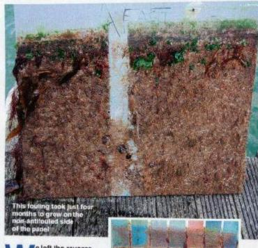
e left the reverse side of each board without antifouling. along with a 20mm border between each block of paint. These areas acted as our control samples.
